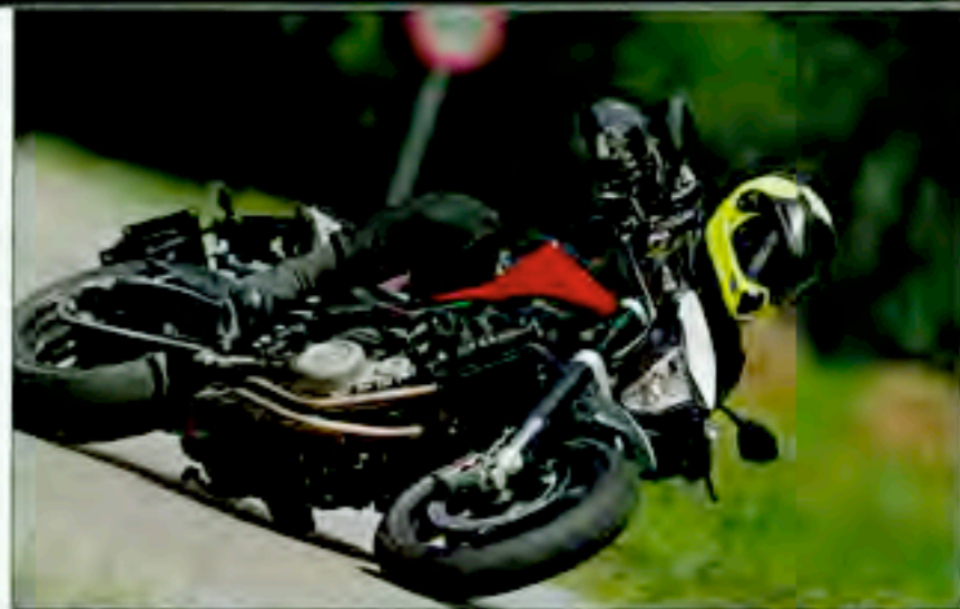
Husky's Nuda R is powered by a pumped-up, 898cc version of the BMW F800 parallel-Twin, but revisions and retuning are so thorough that the two engines seem completely unrelated.
