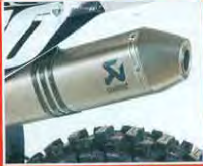
You can't do much better than the stock exhaust system. The Husky comes with a titanium Akrapovic.
