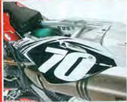
The seat comes off with a single Dzus fastener, allowing no-tool air-filter access.
