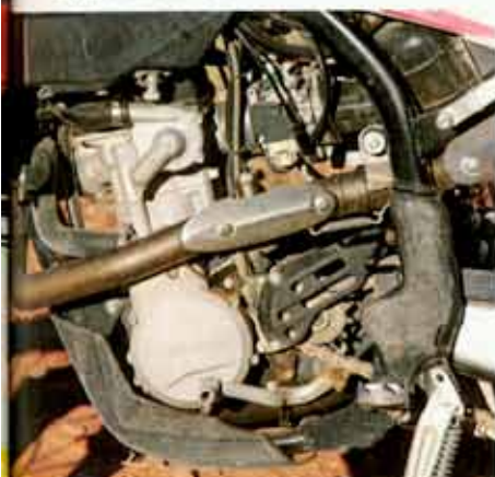
This "little" Husky rips, but at what price? We oddly had an oil pump gear break in ours.
